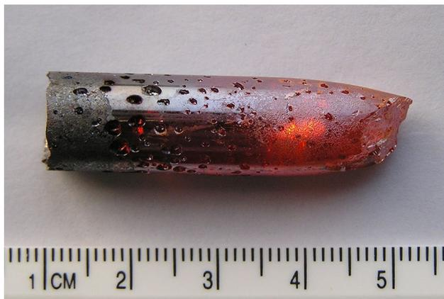
**Fig. 4** Grown boule of  $\text{Pb}_2\text{GeS}_4$  (illuminated from below with white light)
